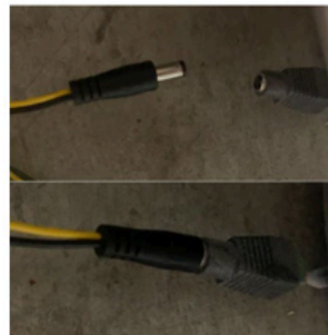
Connecting Harness to LED Port
