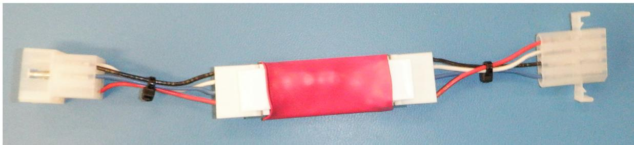
To install a ticket dispenser in an Alan-1 arcade cabinet, plug the signal amplifier into the UCL plug in the back of the machine. There is a UCL plug for each player and is labelled as such:
