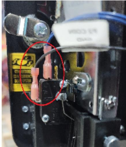
The yellow wires need to connect to the existing wires as seen above; their polarity does not matter. It is best to use a clean wire splice connector, such as crimp-on quick connects, and not anything that would leave exposed wires, as that could result in grounding issues and/or an electrical shock to you or your customers.
