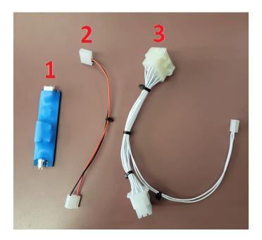
Item 1 is the regulator circuit board while Item 2 is the wire harness that connects the output of the regulator to the TUK. Item 3 is a monitor cable extender that will be either 15 pins for a color monitor or 12 pins for a black and white monitor.
