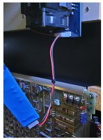
Again, The output wire harness is keyed so it cannot be plugged into the TUK incorrectly. The TUK fan should now receive a regulated 24 volts.
