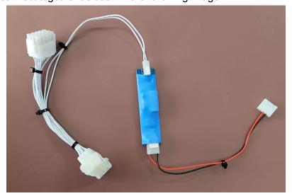
The tail on the monitor cable extender connects to the 2-pin connector on the regulator board while the output wire harness connects to the 4-pin connector on the regulator board. The connectors on the output wire harness are keyed so they cannot be connected to the regulator or TUK incorrectly.
