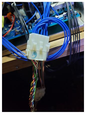
Please note this will be either a 12-pin or 15-pin connector depending on whether you are installing the voltage regulator on a black and white or color monitor.
