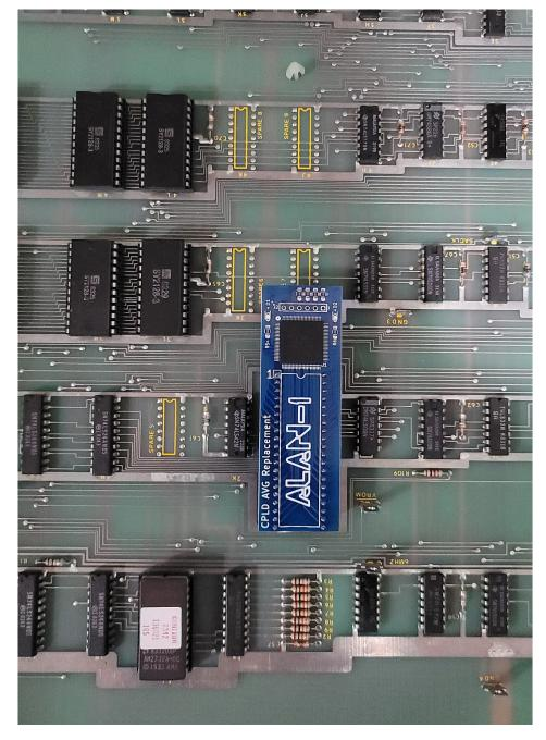
Note that all 40 pins of the AVG replacement should be seated into the 40 positions of the chip socket. **Verify all 40 pins are firmly seated in the chip socket before powering up the PCB.**
