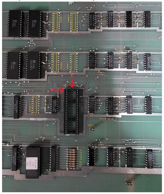
Item 1 above points to the notch in the AVG chip socket. Item 2 above points to position 1 of the AVG chip socket.
