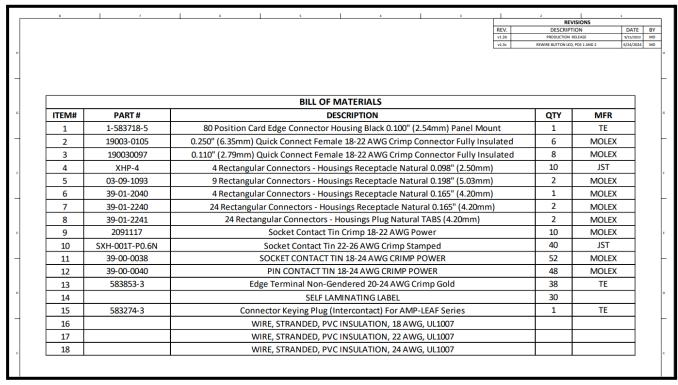
FIGURE 13. 40 PIN WIRING HARNESS BOM
