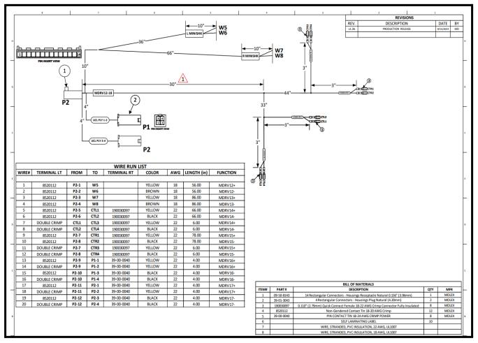
FIGURE 14. COIN DOOR LED & TICKET DISPENSER DIAGRAM
